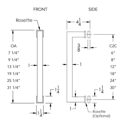
**Installation Notes**: Center to center hole drilling dimension are same as mentioned in column. Diameter of glass hole for installation is 1/2".
